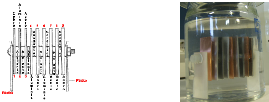
Figure 1: Metal disposition in the corrosion test. In 1 st , 2 nd and 3 rd position we placed aluminium, steel and copper isolated, avoiding formation of galvanic pairs. In positions 4 and 5, we formed galvanic pairs Al-Cu; in positions 6 and 7 Al-Steel, and in positions 8 and 9 we formed the pair Cu-Steel.
