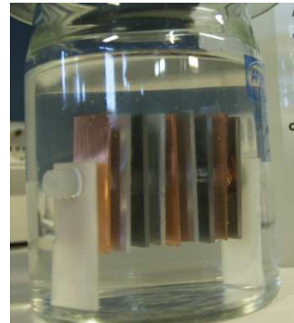
Figure 1: Metal disposition in the corrosion test. In 1 st , 2 nd and 3 rd position we placed aluminium, steel and copper isolated, avoiding formation of galvanic pairs. In positions 4 and 5, we formed galvanic pairs Al-Cu; in positions 6 and 7 Al-Steel, and in positions 8 and 9 we formed the pair Cu-Steel.
